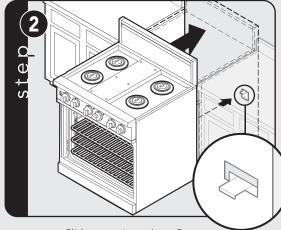
Slide range into place. Be sure anit-tip bracket slides into the anit-tip opening.
